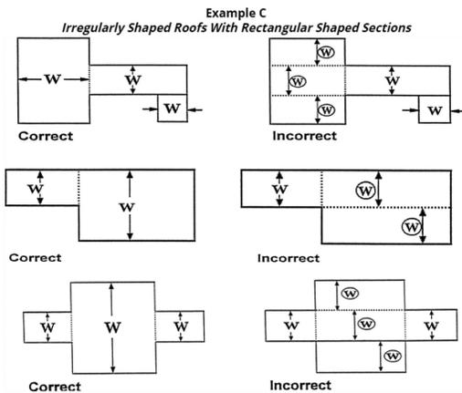
Such roofs are to be divided into subareas by using dividing lines of minimum length to minimize the size and number of the areas which are potentially less than or equal to fifty feet (15.25 m) in width, in order to limit the size of roof areas where the safety monitoring system alone can be used (WAC 296-880-40045(1)). Dotted lines are used in the examples to show the location of dividing lines.
