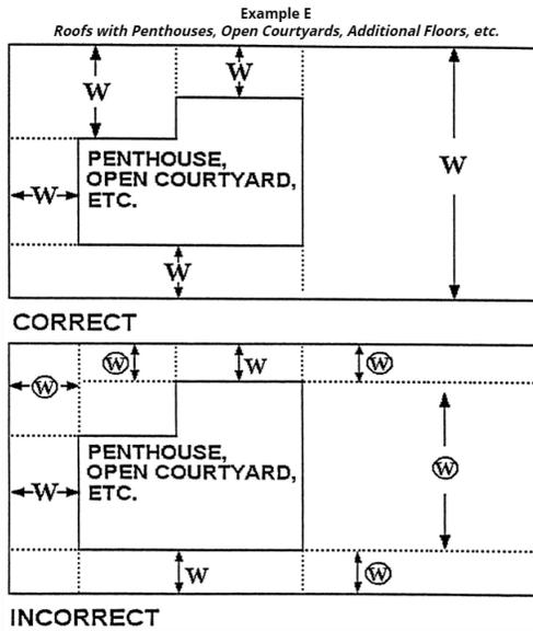
Such roofs are to be divided into subareas by using dividing lines of minimum length to minimize the size and number of the areas which are potentially less than or equal to fifty feet (15.25 m) in width in order to limit the size of roof areas where the safety monitoring system alone can be used. Dotted lines are used in the examples to show the location of dividing lines.
