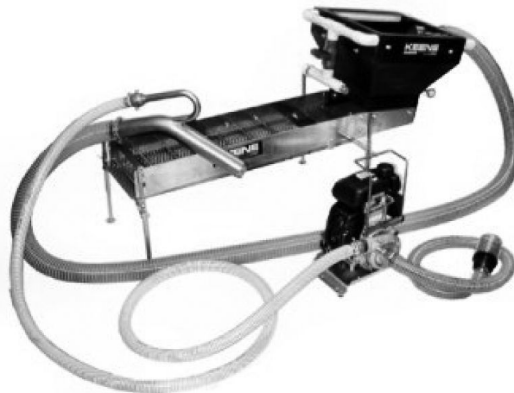
Figure 5: Power sluices/suction dredge combination
