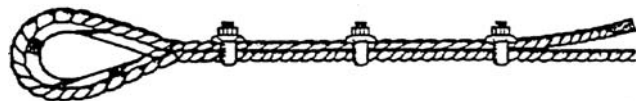
2. WRONG METHOD—U-Bolts on live end of rope. (This will cause mashed spots on the live end of rope)
