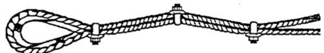
3. WRONG METHOD—Staggered clips; two correct and one wrong. (This will cause a mashed spot in live end of rope due to wrong position of center clip)
