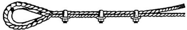
1. CORRECT METHOD—U-Bolts of clips on short end of rope. (No distortion on live end of rope)
