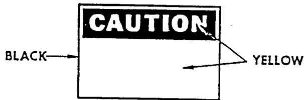
Fig. J-4 Caution Sign
