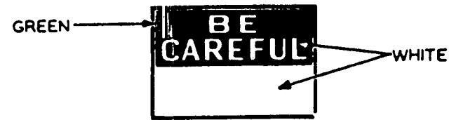
Fig. J-5 Safety Instruction Signs
