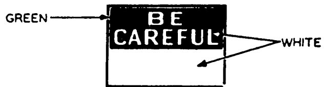
Fig. J-5 Safety Instruction Signs
