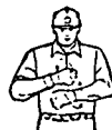
FOR MOBILE CRANES TRAVEL BOTH CRAWLER BELTS IN DIRECTION INDICATED BY REVOLVING FISTS
