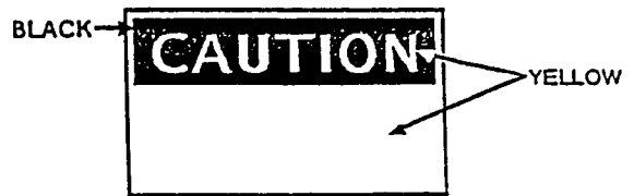
Fig. J-4 Caution Sign
