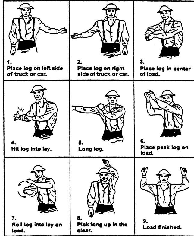
Figure 42: Standard Signals for Loading Logs
