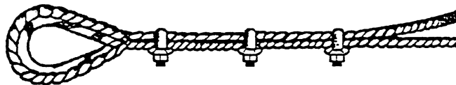
1. CORRECT METHOD—U-Bolts of clips on short end of rope. (No distortion on live end of rope)
