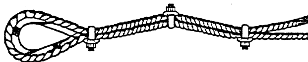
3. WRONG METHOD—Staggered clips; two correct and one wrong. (This will cause a mashed spot in live end of rope due to wrong position of center clip)
