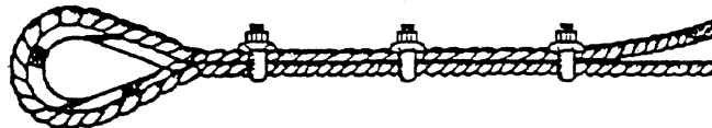
2. WRONG METHOD—U-Bolts on live end of rope. (This will cause mashed spots on the live end of rope)
