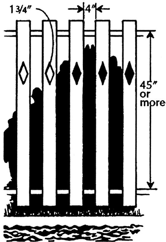
(d). **Vertical Spacing:** If tops of horizontal members are less than 45 inches apart, vertical spacing shall not exceed 1 3/4 inches.
