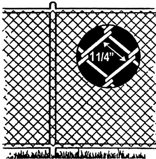
(b). When chain link exceeds 1 1/4 inches square, provide slats to reduce mesh openings to no more than 1 3/4 inches.
