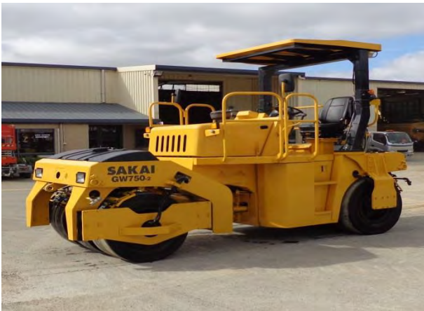
Figure 8. Sakai GW 750-2 pneumatic vibratory intermediate roller.
