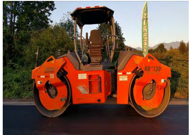
Figure 7. HAMM HD 120 steel wheel oscillatory breakdown roller.
