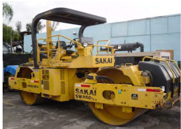
Figure 9. Sakai SW850 steel wheel vibratory finish roller.
