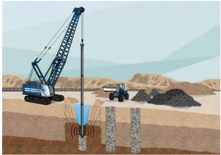
Figure 15. Aggregate Shafts – Example
