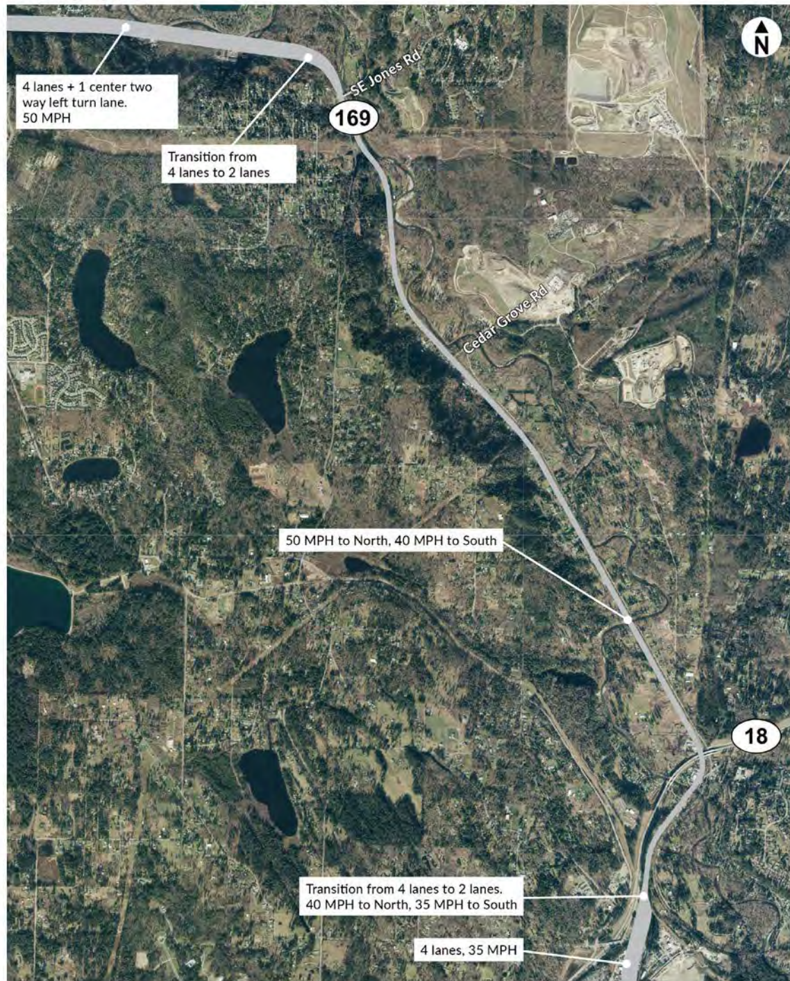
Figure 2. Facility type for SR 169 from Southeast 231st Street to Renton city limits, milepost 14.12 to 21.28 (Source: WSDOT, ESRI)
