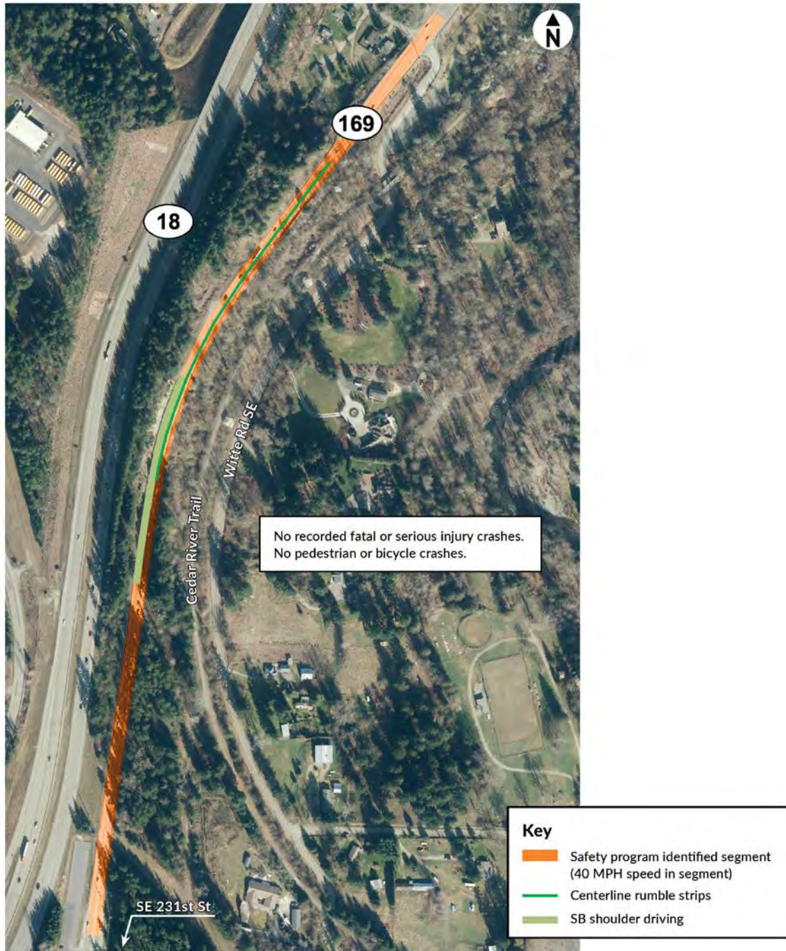
Figure 11: Condition diagram for SR 169 from north of Southeast 231st Street to Witte Road Southeast, milepost 14.29 to 14.95 (Image source: WSDOT SRView via ESRI et al.)
