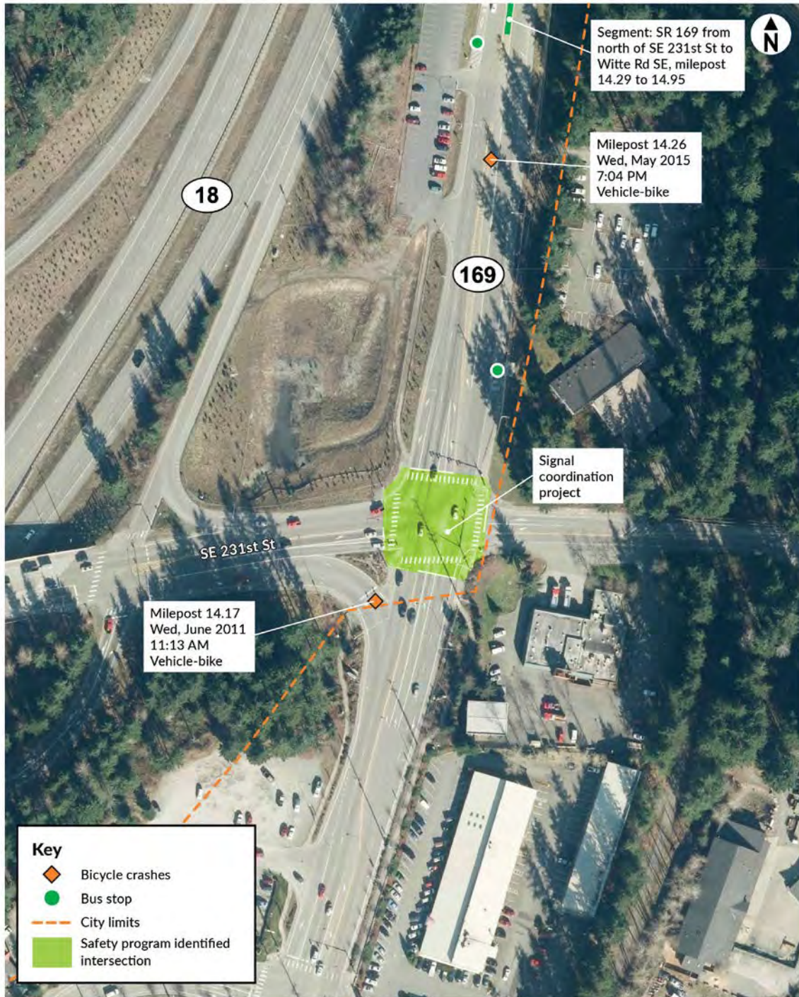
Figure 10: Condition diagram for SR 169 and Southeast 231st Street, milepost 14.17 (Image source: WSDOT SRView via ESRI et al.)
