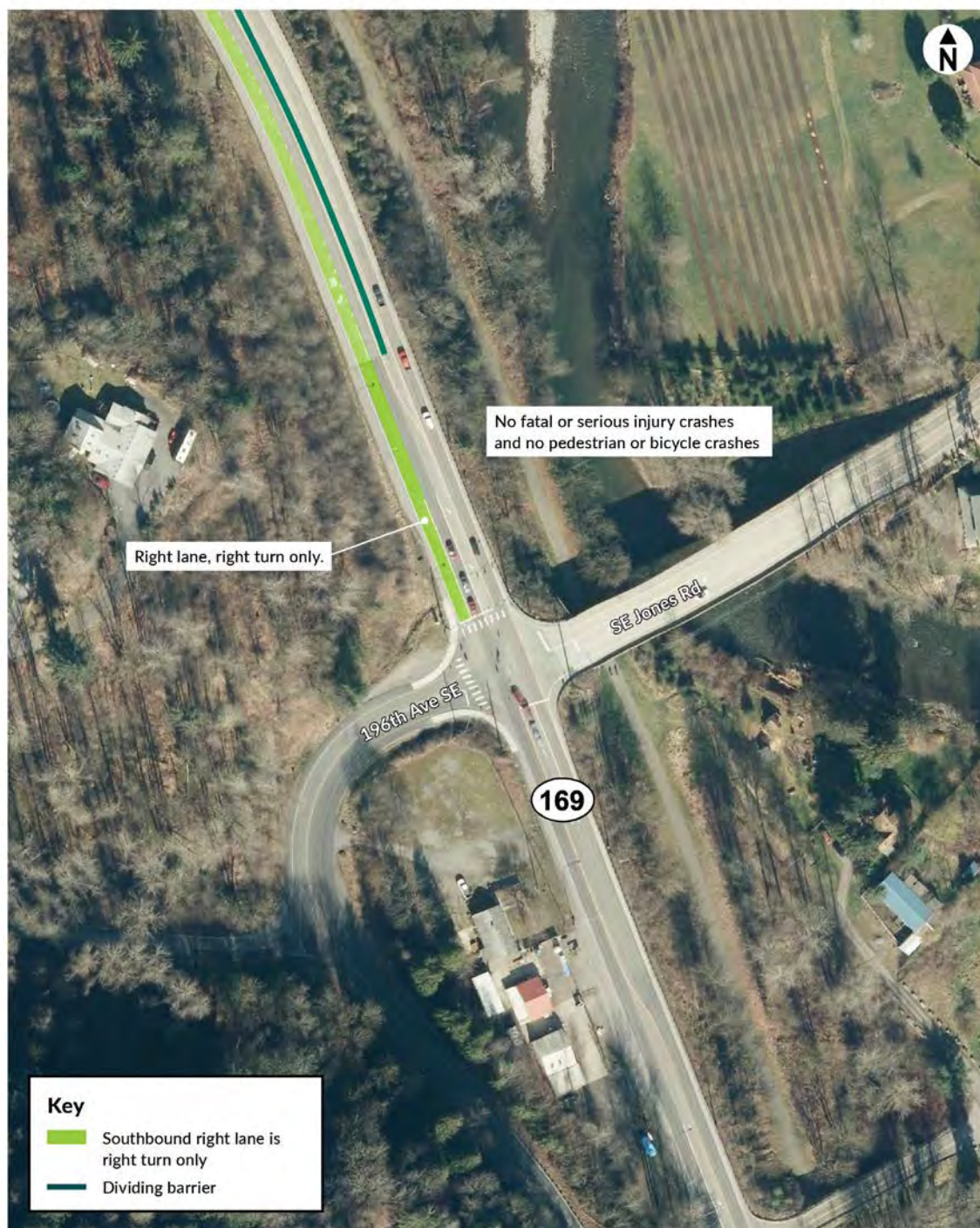
Figure 18. Condition diagram for SR 169 and 196th Avenue Southeast/Southeast Jones Road, milepost 19.22 (Image source: WSDOT SRView via ESRI et al.)
