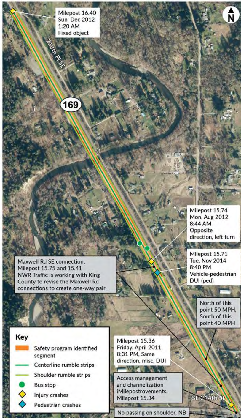
Figure 12: Condition diagram for SR 169 from Southeast 214th Street to 218th Place Southeast, milepost 15.34 to 16.40 (Image source: WSDOT SRView via ESRI et al.)
