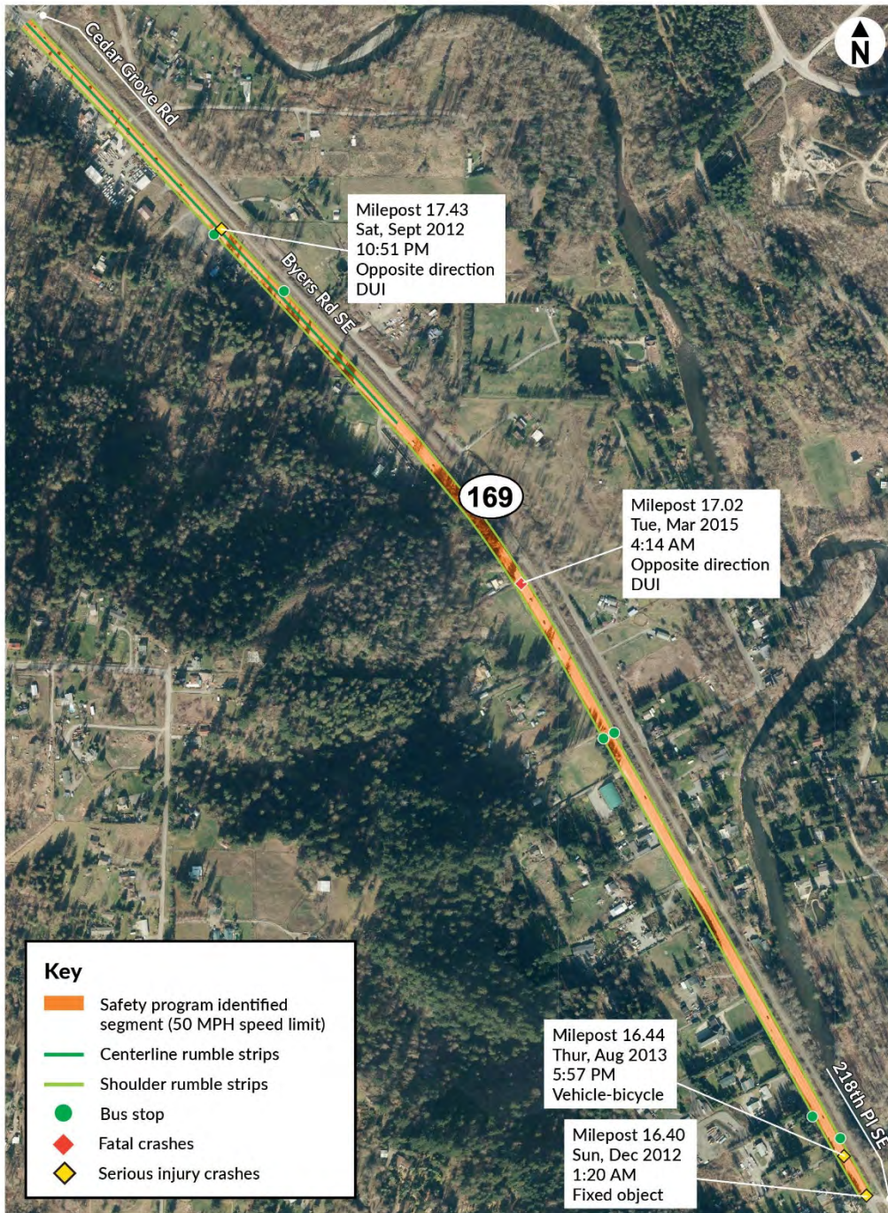
Figure 13: Condition diagram for SR 169 from 218th Place Southeast to Cedar Grove Road, milepost 16.40 to 17.68 (Image source: WSDOT SRView via ESRI et al.)
