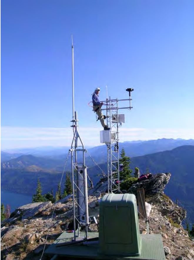
Figure 5: Typical ridgetop RAWS site for wind, temperature, and humidity data
