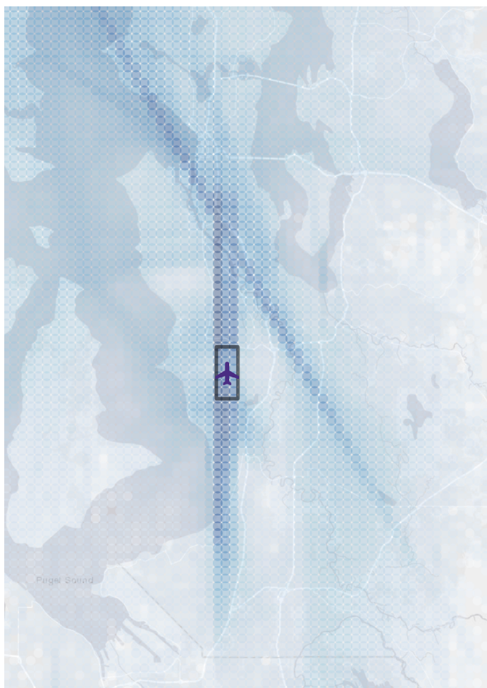
Figure 11: The gridded spatial distribution of the number of arriving and departing flights that are below 750 m in altitude in the year 2018 for the Seattle metropolitan area.
