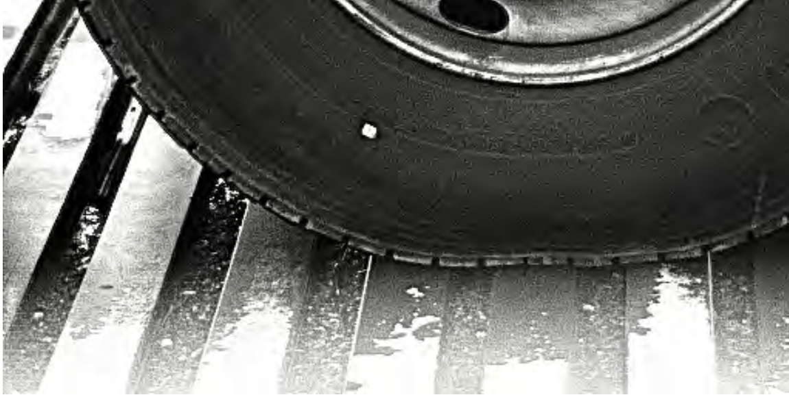
Figure 5-20 Frame from high-speed video recording of a car-carrier truck front tire passing over east-side large expansion joint center beams.
