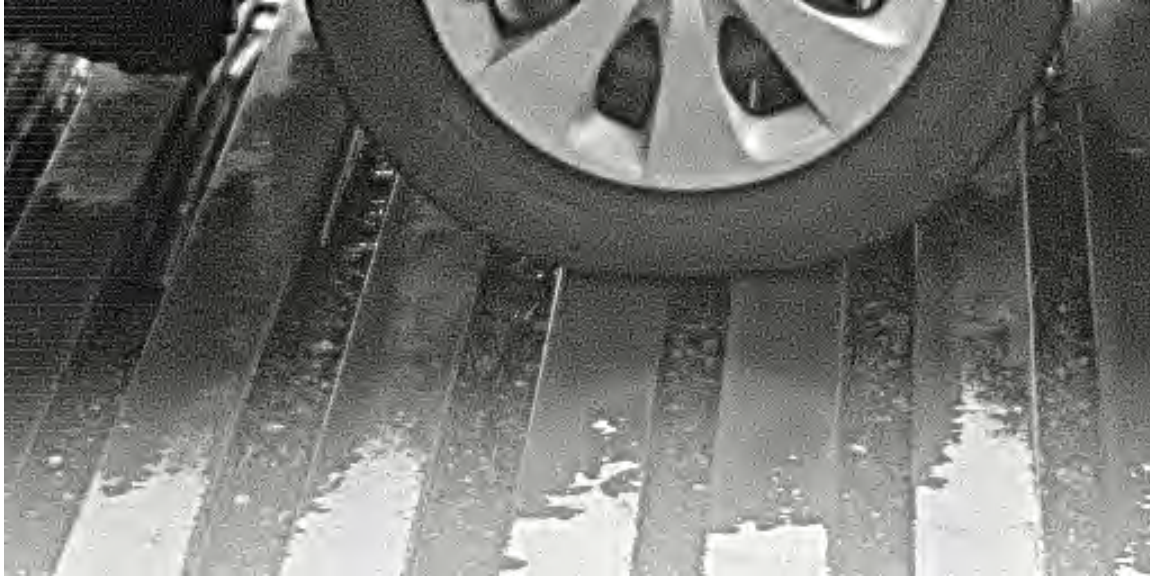
Figure 5-16 Frame from high-speed video recording of Toyota Prius front tire passing over east-side large expansion joint center beams.
