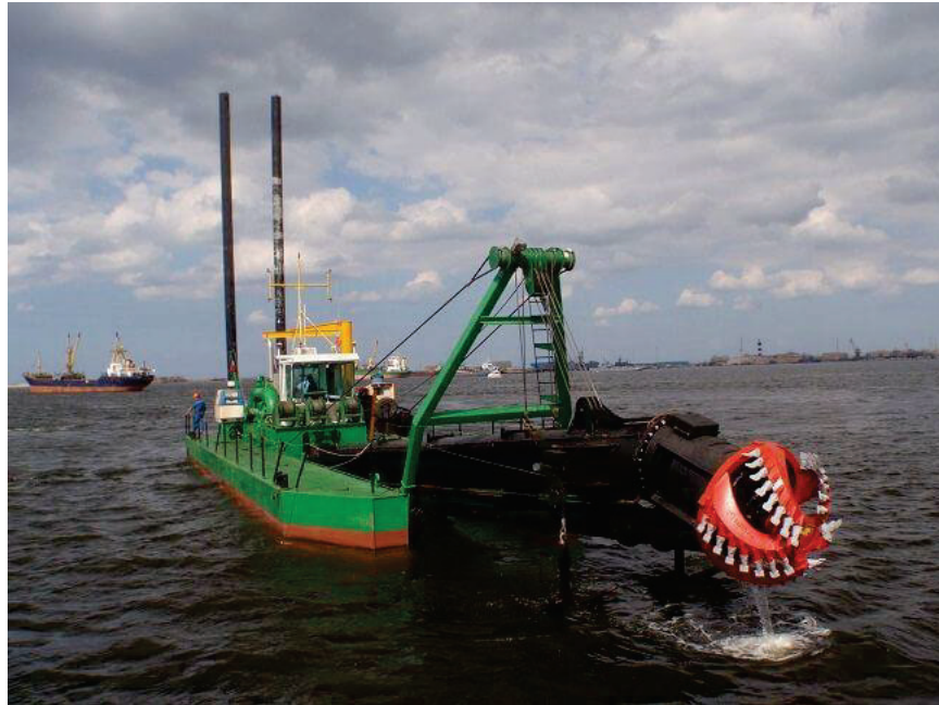
Figure 2 Example of Hydraulic Dredging Barge with Cutterhead Shown in Red
