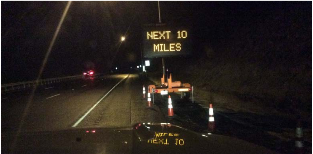
Figure 9. Variable message signs used to warn I-90 motorists of the potential for elk to be on or near the freeway.
