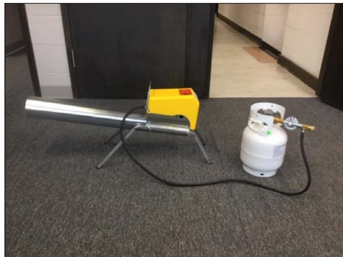
Figure 7. Propane powered noise cannon used by WSDOT to frighten elk near I-90.
