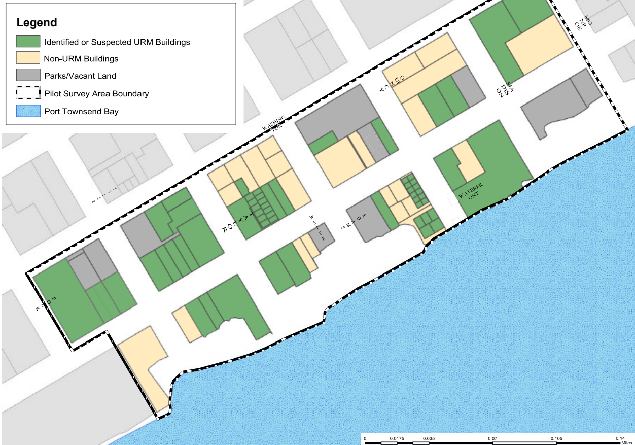
Figure 4-2. The survey area includes 30 identified URM buildings, along with two suspected URM buildings for which construction material could not be confirmed.
