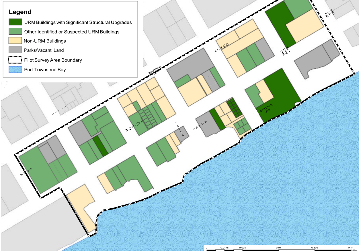
Figure 4-3. Of the 30 identified URM buildings, 5 have undergone extensive seismic upgrades.
