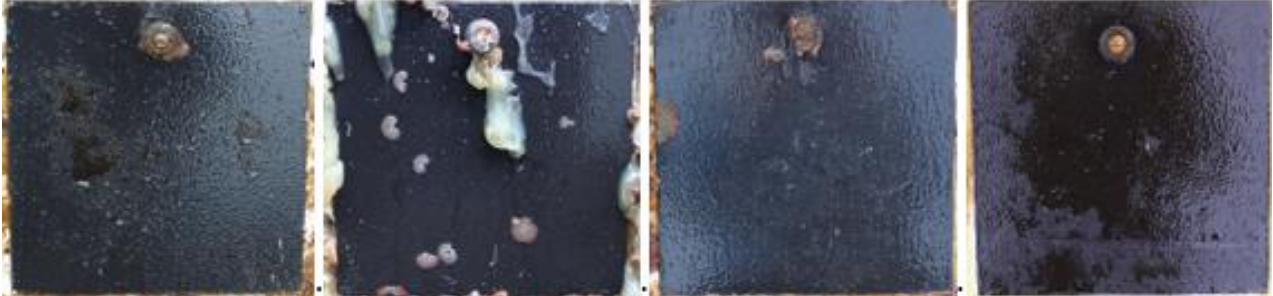
Figure 13: InterSleek® 1100 SR, PIN 10 – from Port Orchard, Gig Harbor, Anacortes, and Seattle – January 2024 (left to right).
