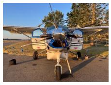
Photo 10: Front view of a Daher Kodiak 100 light fixed-wing aircraft. Photo by Aviation Section.
