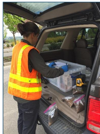
Photo 2: Ecology staff screening arsenic levels with an XRF tool.
