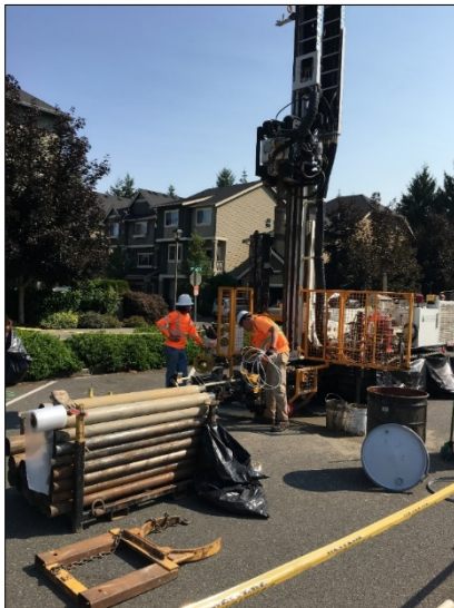
Figure 59: Consultants conduct soil and groundwater sampling in King County's Lower Issaquah Valley to identify potential sources of groundwater contamination. Photo credit: Mike Warfel, Washington State Department of Ecology, August 2018
