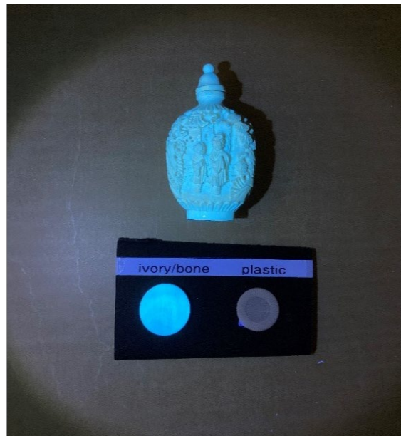
Figure 3. This carved opium bottle was received via a bidding process by WDFW detectives. The bottle was scanned under a UV light, and it was determined that the bottle was made from ivory/bone. Photo provided by WDFW Police.
