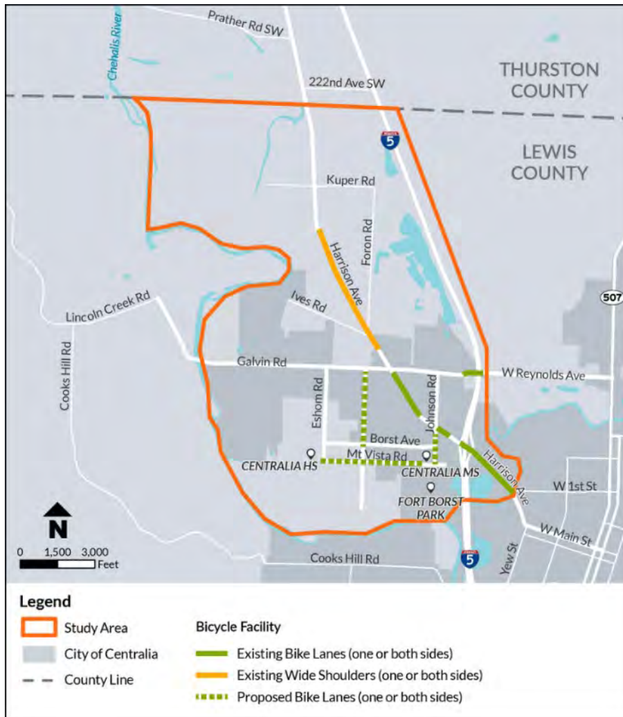
Figure 7-3: Existing and Proposed Bicycle Facilities
