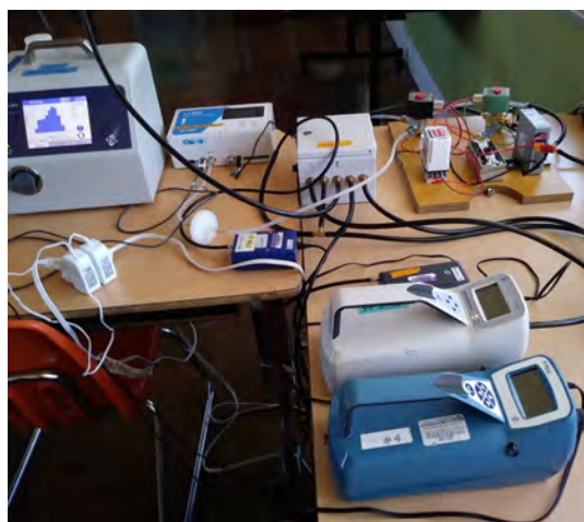
Figure 4 - Instrument arrangement for indoor and outdoor air sampling.
