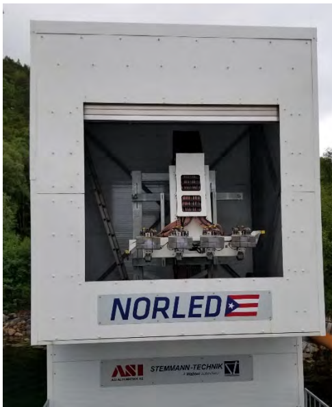
Figure 9: Stemmann-Technik First Generation Horizontal Pantograph RCS
